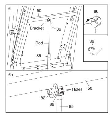
7. Remove the Spring Clip (86) from the lower end of the Gas Spring (85). Press the lower end of the Gas Spring onto the Mount (82) on the bracket in the center of the Base (80). Note: It may be necessary to pivot the Frame (not shown) forward or backward slightly (see HOW TO LOWER THE TREADMILL FOR USE on page 15).
